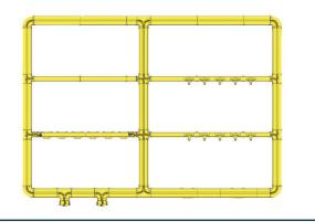
Typically used to create a physically redundant pathway in central offices or high reliability data centers, this design also provides more routing flexibility and reduces cable congestion. A larger, higher capacity channel forms a perimeter around the FDF and Network Element Bays areas to provide a diverse route for cables leaving the FDF. Smaller channels are used to create pathways between the main runs allowing access to the individual equipment bays.
